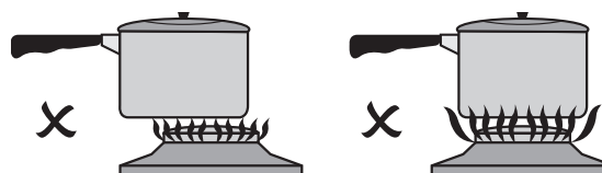
Incorrect – pan not centred.
